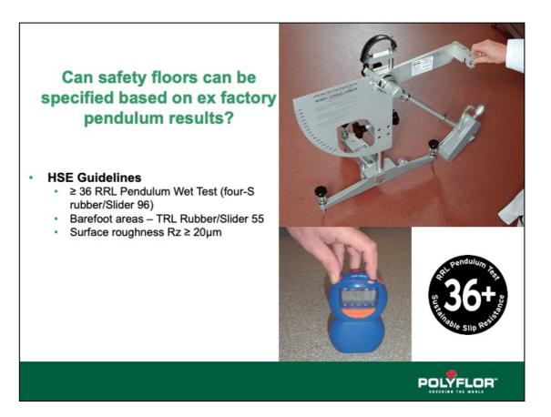
The pendulum test is recommended by UKSRG and the UK Health and Safety Laboratory as the most suitable 'in-situ' test for measuring slip resistance of floor coverings.
