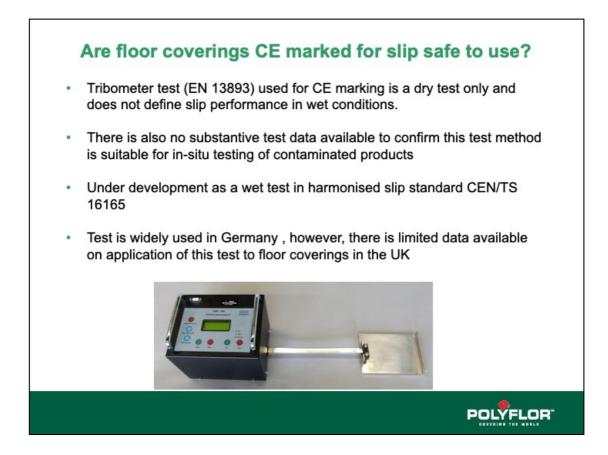
A tribometer test known as the GMG test is used to measure dry slip as part of CE marking floors to EN14041 standard. Floors that meet the required threshold are classified as DS within the CE mark. It is sometimes misunderstood that the DS classification means that the floor covering is slip resistant, however, it should be made clear that this classification applies to dry slip only and has no relevance to wet slip.
