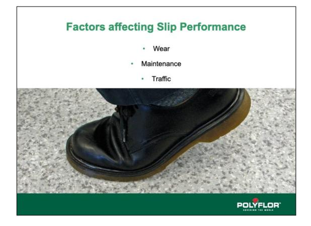
The previous slide outlined ex factory slip performance test results. However, when a floor covering is installed it will be affected by the way it is used in surface, i.e. walking , cleaning regimes, dirt build up and other uses in the area. These can lead to wear of the surface which can in turn affect the slip performance.
