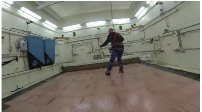
Figure 1. A participant walking down a wet ice slope of 13 degrees in WinterLab while wearing the test boots.
