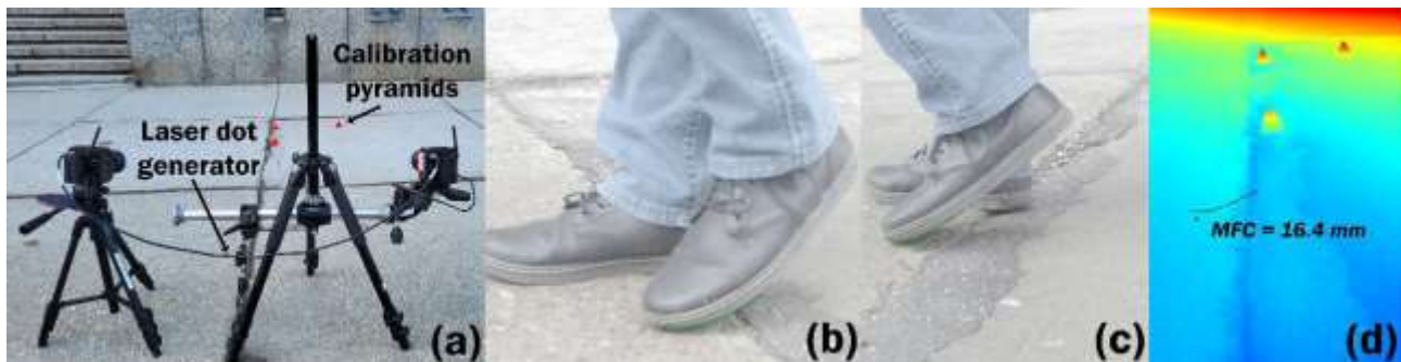
Figure 1. The dual-camera setup (a), the video images of a pedestrian recorded by the left (b) and right (c) cameras. The green dotted lines show the selected matched areas on the edges. The reconstructed 3D shoe edge (black dotted line) overlaid on the 3D model of the sidewalk (d). The red dot on the top dotted line and the black dot on the sidewalk show the lowest point on the shoe edge and its closest neighbour on the sidewalk, respectively (a case result, MFC = 16.4 mm).
