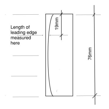
The slider edge length was measured at the mid-point between the centre and the end of the long axis of the slider rubber i.e. approximately 19 mm from one end of the slider. All the length measurements were made in the same way.
